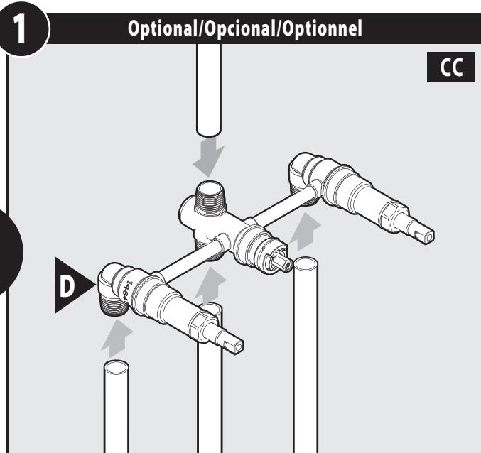
If soldering copper tubing (CC) into valve (D) insert  $\frac{1}{2}$ " copper tubing into the hot and cold water inlets and the shower riser and tub drop outlets.
