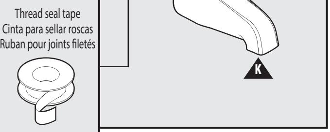
IPS (threaded) spouts are designed to screw onto a pipe with 1/2 inch male pipe threads. To determine the proper pipe length, measure from the inside elbow shoulder to the wall (y) and from the threaded adapter inside of the tub spout to the base of the tub spout (x), then add 1/4". Place thread seal tape around the pipe threading and a sealant (plumbers putty or caulk) around the base of the pipe to prevent leaking behind the wall. Thread the tub spout onto the pipe until flush with the wall.
