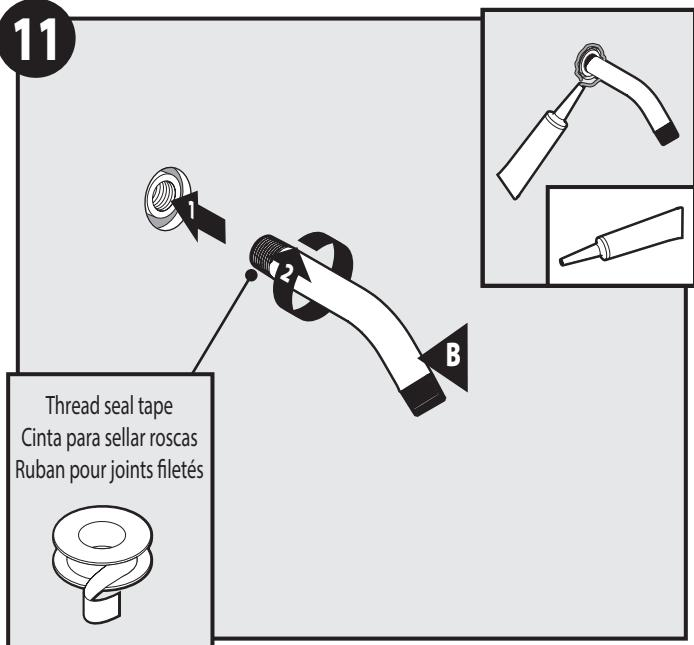
Wrap thread seal tape onto the shower arm (B) threads clockwise. Thread shower arm (B) clockwise into shower arm elbow in wall. Apply sealant to the area surrounding the wall area and pipe.
