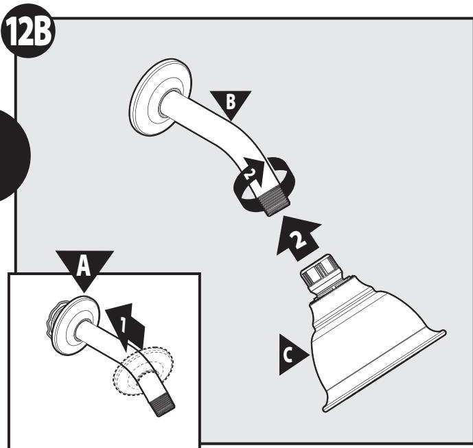
**Metal Shower Ball:** Slide Shower Arm Escutcheon (A) over the Shower Arm (B). Wrap thread seal tape around threads at bottom of Shower Arm (B). Remove any debris from Shower Arm to ensure proper flow. Thread Shower Head (C) onto Shower Arm (B).
