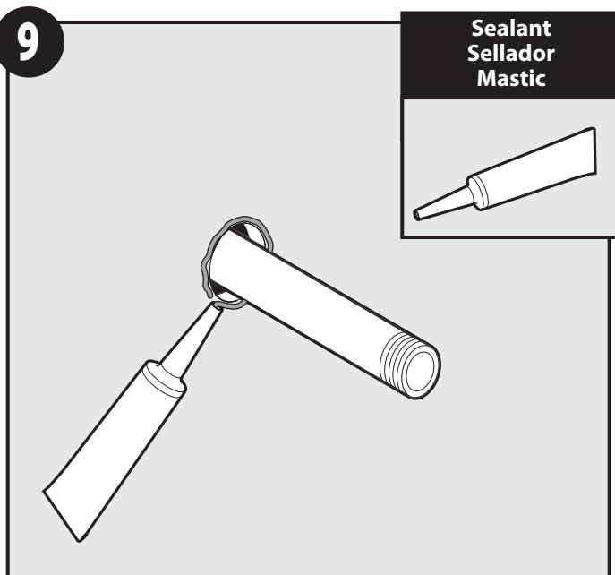
Apply a sealant between the wall opening and the pipe.
