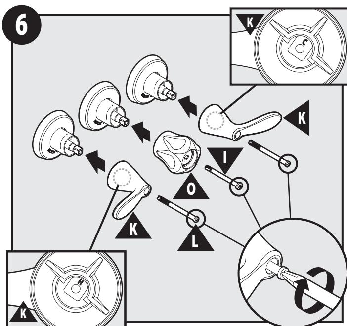
Slide on Handles (K) and Diverter Knob (O), hot and cold knob Handle Screws (L) and diverter knob screw (I). Tighten all screws clockwise with a Phillips screwdriver.
