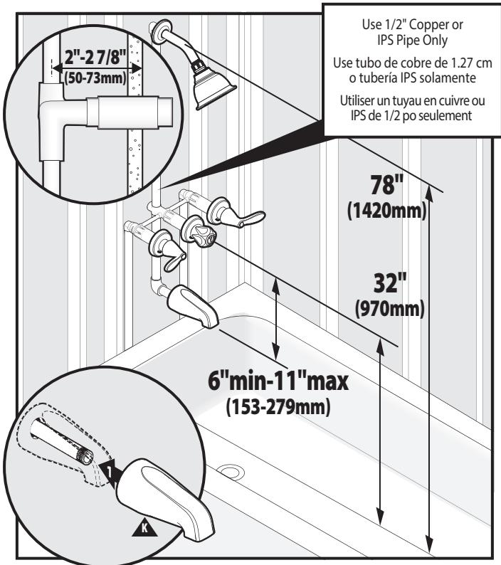
For ease of operation and best performance, install the valve body 32" above the floor and the shower arm at 78" above the floor. The tub spout can be installed between 6" and 11" below the valve body using  $\frac{1}{2}$ " copper tubing or the equivalent to  $\frac{1}{2}$ " brass pipe size material. No more than one elbow is recommended.
