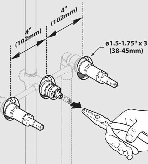
Using needle nosed pliers pull diverter stem out to the open position.
