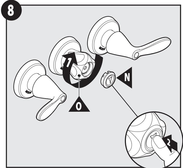
1. Rotate Diverter Knob Handle (O) clockwise until it stops.
