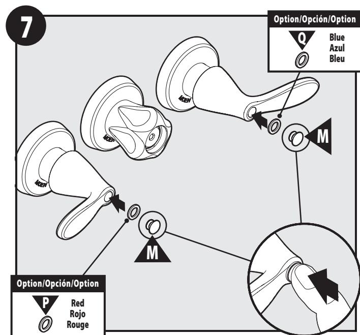
If desired, the blue cold temperature indicator (Q) and the red hot temperature indicator (P) can be installed onto the handles and are held in place by the handle caps (M). If no temperature indicators are wanted, install the caps (M) into the handles as shown.
